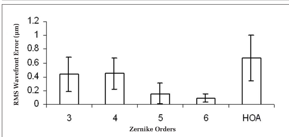
Figure 2. Root-mean-square (RMS) wavefront error of 3rd to 6th order and total higher order aberrations (HOA) in eyes with monofocal IOLs (pupil diameter=6 mm).
